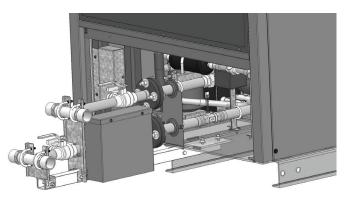
Figure 2-10 Multi-Manifold Assembly
