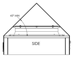
Figure 2-6 Water heater and forklift fork position
